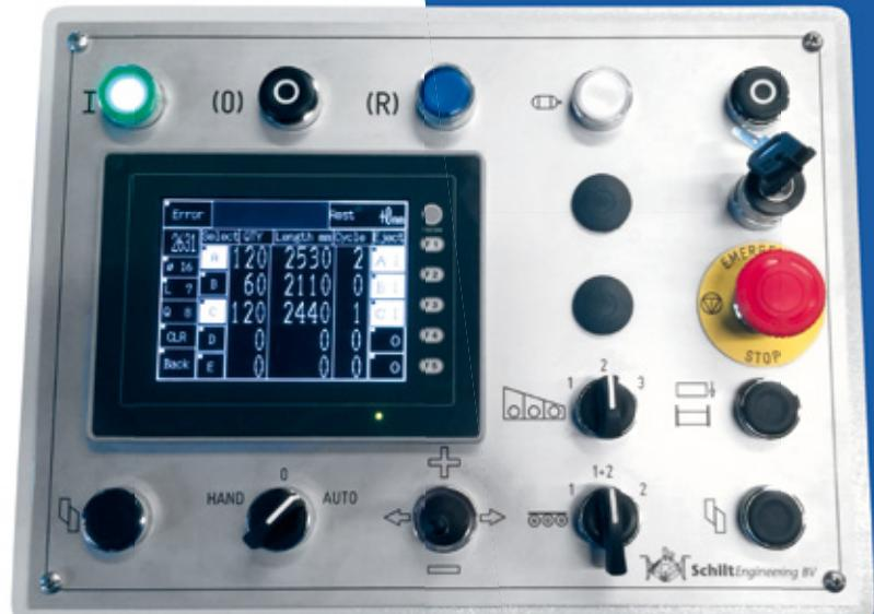
UK Modern controls with touch panel, automatic cutting program and possibility to attach barcode scanner. Optional also with PC control for data transfer from office ERP systems.
