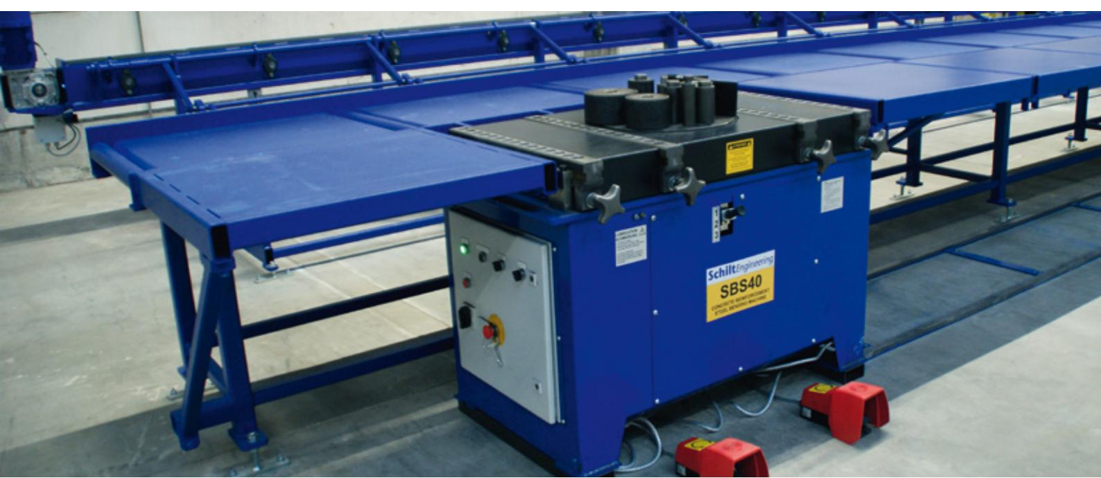
🇬🇧 Standard version with collecting boxes beside the eject track, optional versions with integrated rebar benders or with automatic double bending line.
