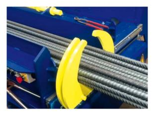
To bundle the positions, a sliding hydraulic clamp can be provided at the end of the roller conveyors (optional).
