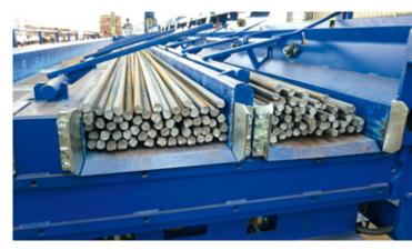
Roller conveyors electrically driven. The high-quality roller coating guarantees the highest level of noise insulation.
