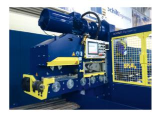
Feeding and measuring system with servo drive.
